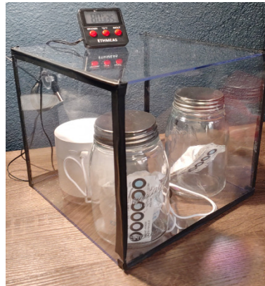
Figure 1. An acrylic box with dimensions of 9.44" x 9.44" x 9.44" housed as the first iteration of the chamber.
