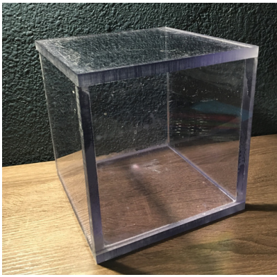
Figure 3. Polycarbonate sheets made up the second iteration of the chamber. With dimensions of 8” x 8” x 8”
