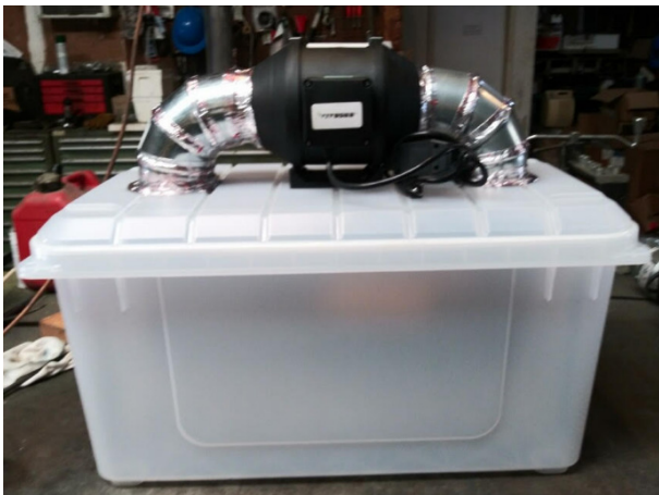
Figure 4. The constructed tote box with a Vivosun 4” inline tube fan attached alongside ducts.
