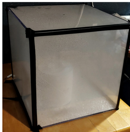
Figure 2. The acrylic chamber in use during the efficacy tests of the various desiccants
